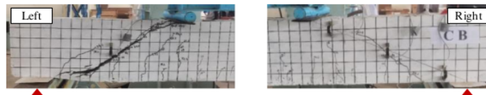
Figure 5. Crack pattern of CB
